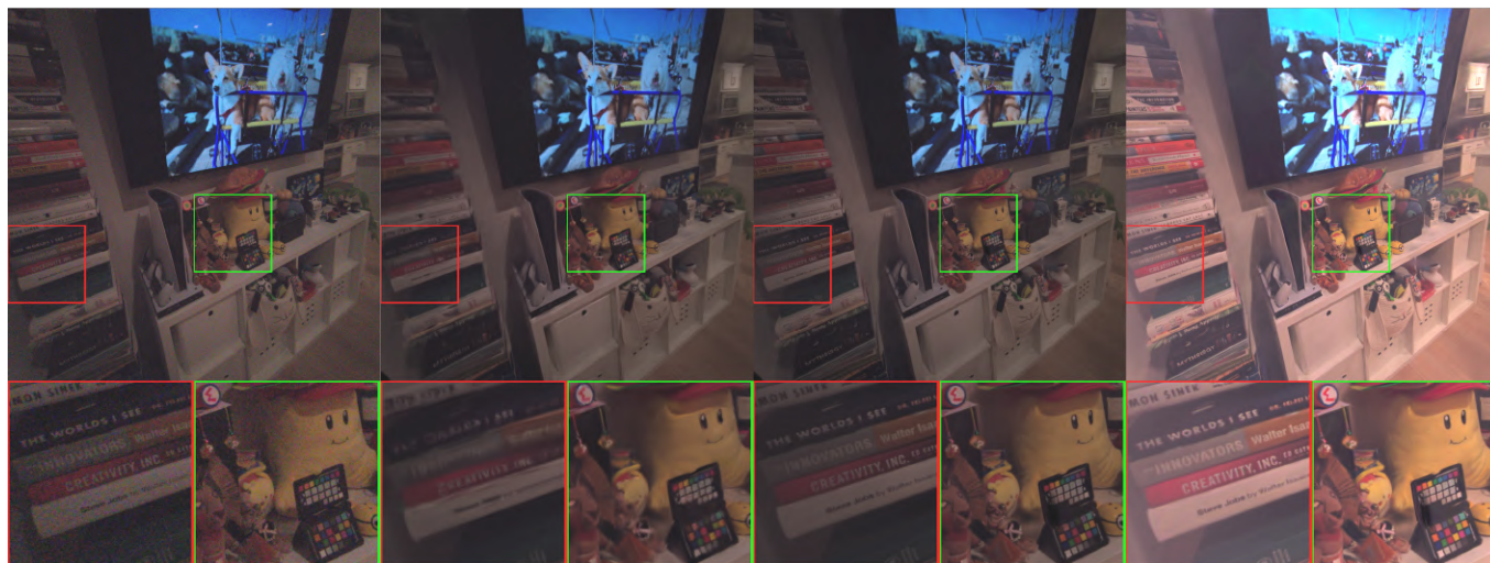
Fig. 1. A comparison (from left to right) of (a) the raw camera held-out reference image, (b) the reconstructed view from a vanilla Gaussian-splatting algorithm using device calibration, (c) our reconstruction result using our proposed system, and (d) our reconstruction rendered with lifted dynamic range. We adjust the gamma of all comparisons for better visualization. Egocentric video may contain challenges in image quality due to high speed head motion and the form factor constraint. Our proposed system can recover photoreal scene reconstruction from the egocentric input videos with noises and heavy rolling-shutter effect. Note the improved clarity on the text in the low-light image areas due to our correct handling of rolling-shutter during both steps in visual inertial bundle adjustment and Gaussian-splatting. As a result, we can render the videos with higher dynamic range and further boost the details.
